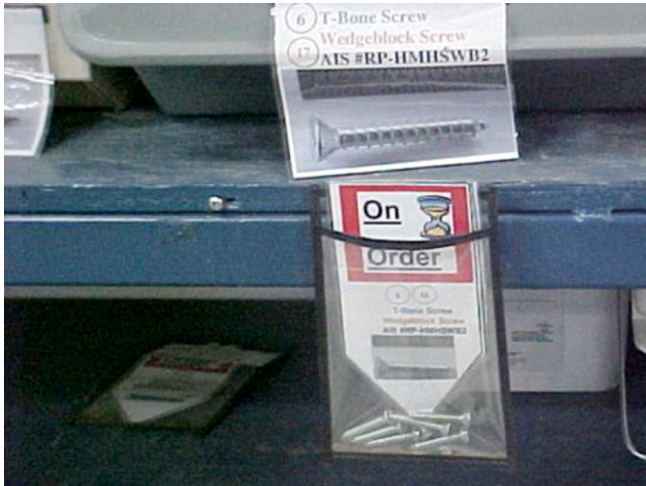
Figure 6. A kanban card used in an institutional furniture factory. The card will signal the upstream process that inventory needs to be replenished.
