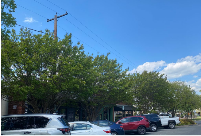
Figure 8. An example of appropriately sized trees (crape myrtles) planted under distribution utility lines. (Photo by Eric Wiseman.)
