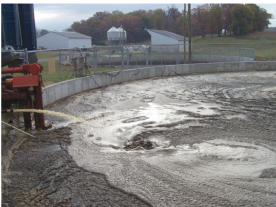
Figure 2. Chemical application to manure in storage tanks for phosphorus removal; struvite recovery reactor from manure to recover phosphorus.
