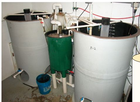
Figure 2: Recirculating rotifer production system.
