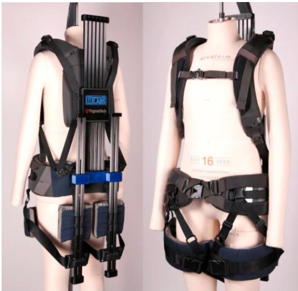
Figure 2: Front and back view of Virginia Tech and Lowe's passive Exoskeleton (Alemi et al. 2019).
