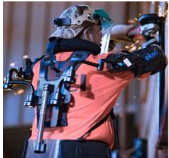
Figure 3: A person using an angle grinder with support from a passive exoskeleton (Olar, Leba, and Risteiu 2021).
