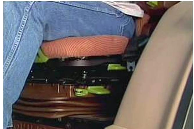
Figure 1: Improved seat cushions designed to insulate operators from vibration (Grisso et al. 2010, 2)
