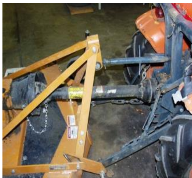
Figure 4: A mower attached to a tractor via a PTO (Murphy 2022)
