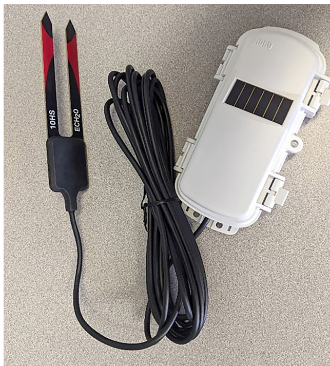
Figure 3. A pronged volumetric water content sensor attached to a remote data collection device.
