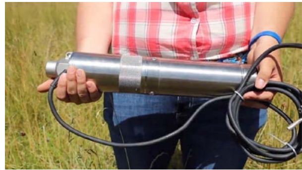
Figure 11. Photo of Small Submersible Positive Displacement Pump
