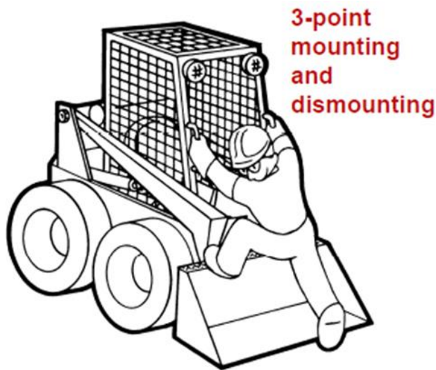
Figure 2. Always have three points of contact for entering and exiting the skid steer. Illustration courtesy of Penn State Extension.
