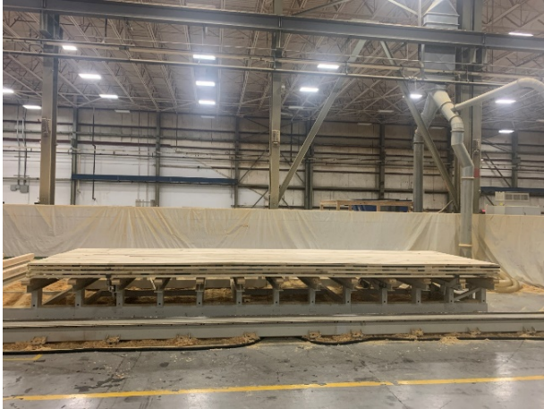
Figure 5: CLT panel pull-out form press and ready for CNC work.
