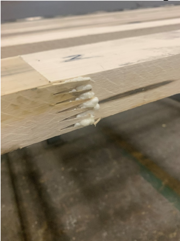
Figure 2: Fingered jointed lumber.
