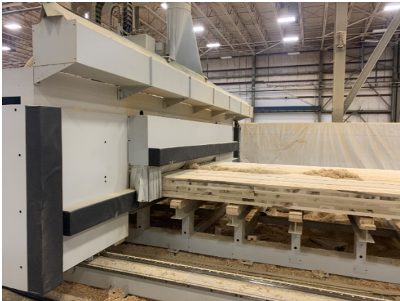
Figure 6: CNC machine working on the panel to cut into final dimension.
