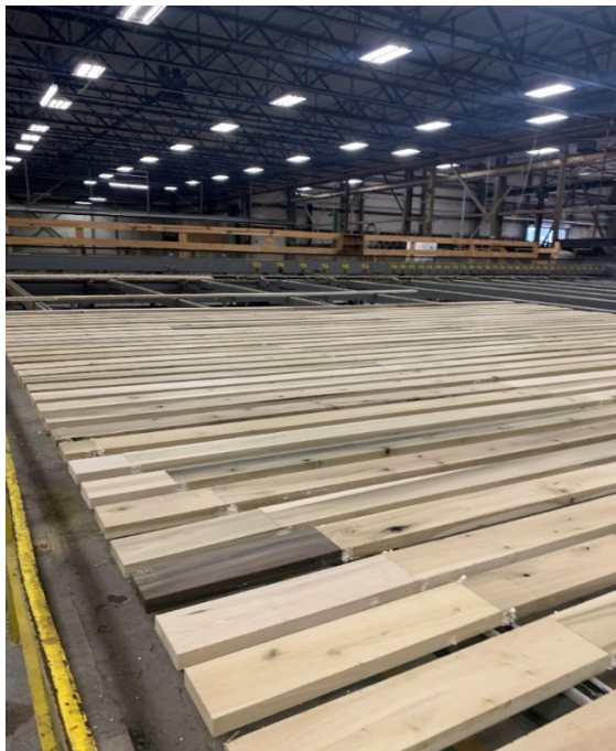
Figure 3: Lumber cut to CLT lengths after finger jointing.
