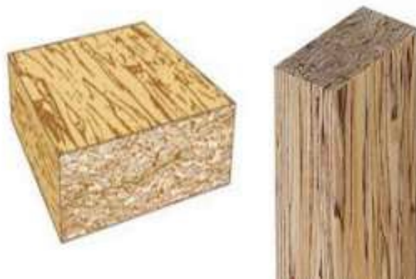
Figura 5: Madera de fibra paralela (PSL).(CWC, 2021d; Naturally Wood, 2021b).
