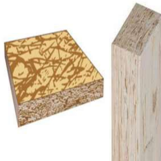
Figure 3: Madera de fibra laminada (LSL) (CWC, 2021b; Naturally Wood, 2021a)
