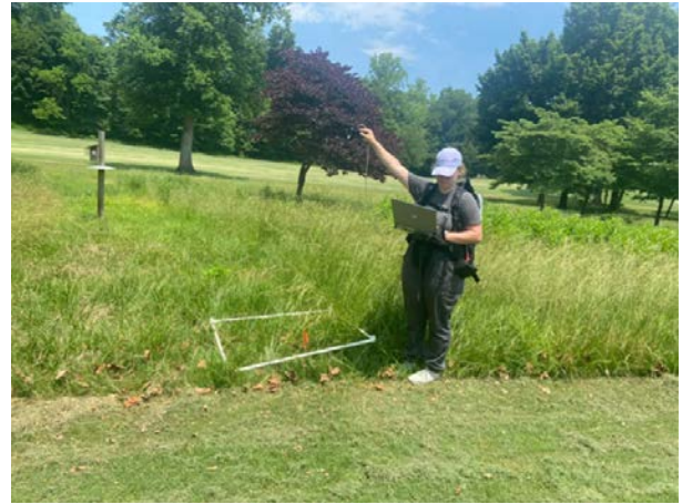
Figure 6. The spectrometer in use (backpack) at a golf course, collecting light reflectance. Photo by Joseph Leo.
