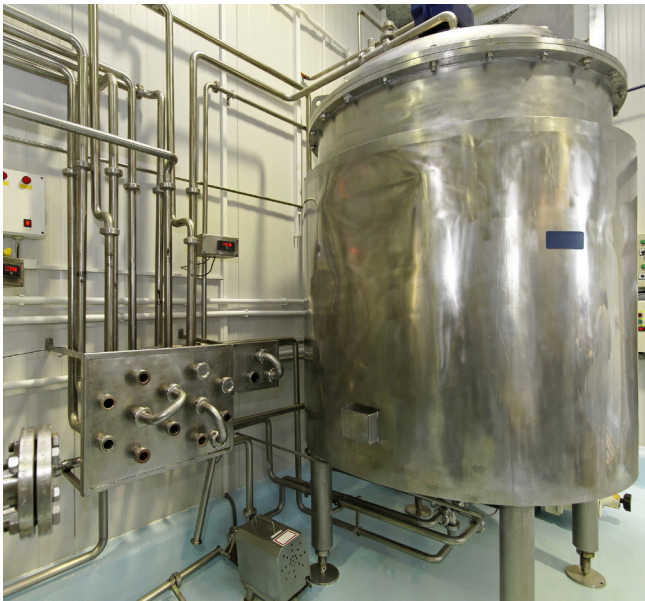
Figure 3. This is an example of a bulk or batch pasteurizer typically used to pasteurize product all at once and/or after being packaged. (Photo courtesy of Markobe from Adobe Stock)
