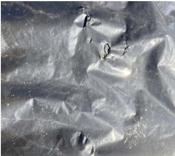
Figure 6. Deer damage on a UV-treated silage tarp. (Shawn Jadrnicek, Virginia Cooperative Extension)
