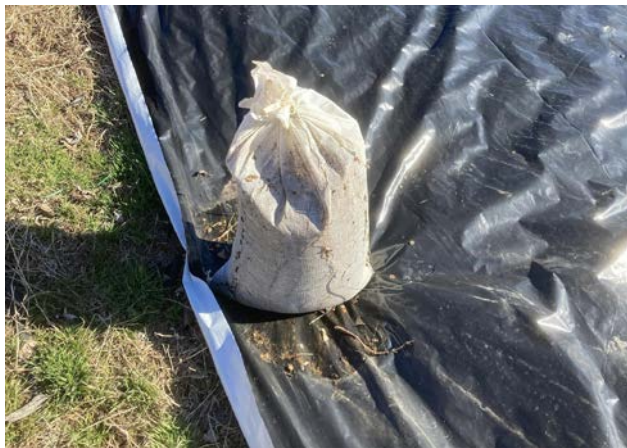
Figure 2. This 10-15 lb. bag used for securing occultation or solarization tarps is not UV resistant and will photodegrade within a year. (Shawn Jadrnicek, Virginia Cooperative Extension)
