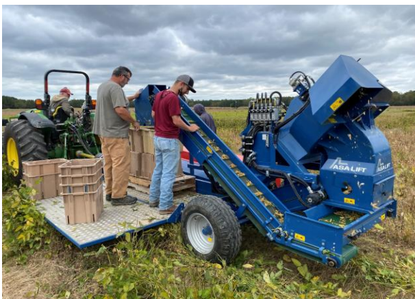
Figure 2. ASA-LIFT GB-1000 mechanical snap bean picker harvesting edamame.
